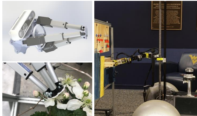
Fig. 5. (left) soft parallel end effector designed for BrambleBee pollination; (right) the linear vertical lift, Dynamixel servo based manipulator, and compliant gripper developed by the PI's student competition team.
